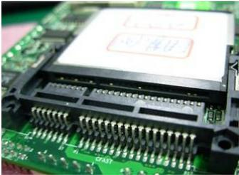
Installing the CFAST in the back of the board.
