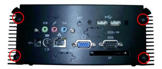
6. Put on HDD driver and lock the screw.
