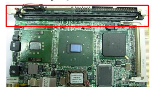
4. Press down the memory module then check DIMM holder hook well.
